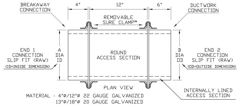
FABRICATE IN ACCORDANCE WITH LANGDON'S DUCT CONSTRUCTION STANDARDS
